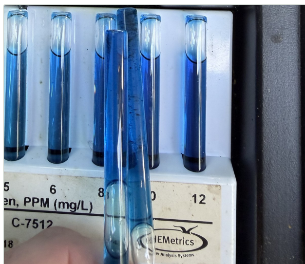
Fig. 2 — Field sample ampoule color-matched between the 8 and 10 mg/L standards.
